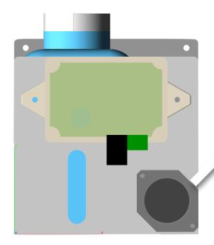
Connect one end of the vinyl tubing to the pump outlet and the other end to the Tee barb as shown. Cut vinyl tubing to length if necessary.
