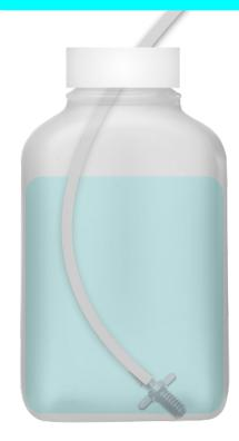
Unscrew the cap and lift out the intake tubing. Remove the bottle. Fill with any White Vinegar. Replace the bottle with the label facing the back and screw on the lid. Make sure that the intake pipe is at the bottom of the bottle. The 16 oz (500 ml) reservoir can last for months. More on website: <u>https://draindrizzler.com/care/</u> We suggest you check the vinegar level every couple of months, but particularly before the start of the Summer algae season.
